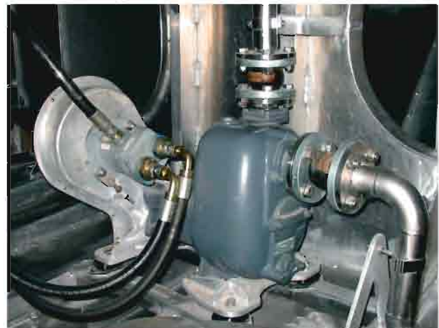
带发动机液压驱动的J 2-180, 用于捕鱼船 J 2-180 with hydraulic motor on a fishing boat
